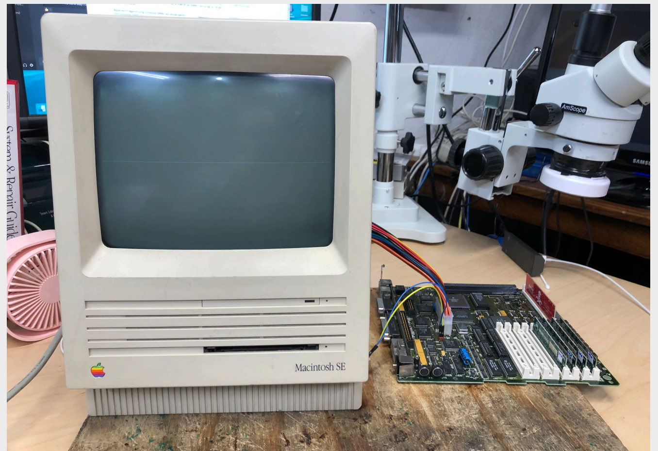
An SE/30 logic board connected to its chassis via an ATX extension cable. This allows you to easily inspect components and test connections without needing to re-assemble the entire computer.
