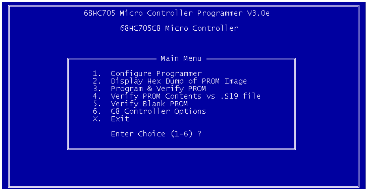
Figure 23 - 68PROG05 Main Menu configured for the 68HC705C8 micro controller
